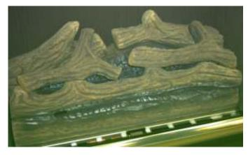
8.1.4 Place the remaining log to the right hand side of the fuel bed to bridge the front and rear log pieces. The stubby branch should nestle down and be located in the notch on the right of the rear log piece. The other end of the log shall come to rest on the branch stub
