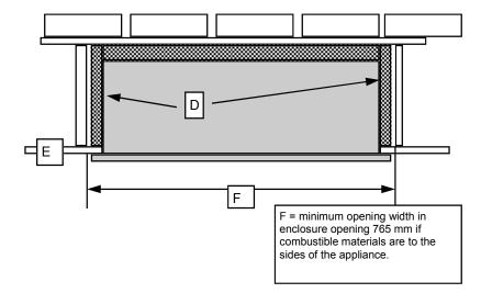
rear of the appliance location shall be protected with rigid non combustible insulating board or 50 mm thick rock wool or similar.
