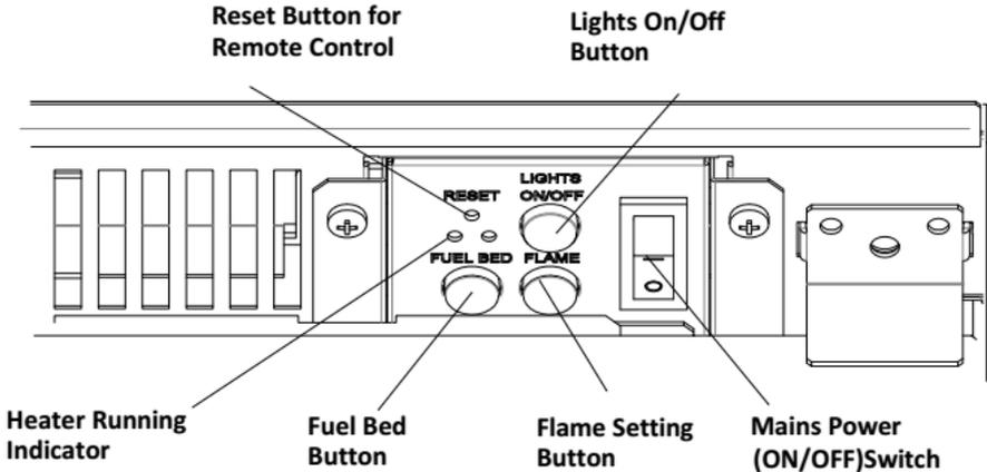
6a.1 The manual buttons are located at the upper of the appliance.
