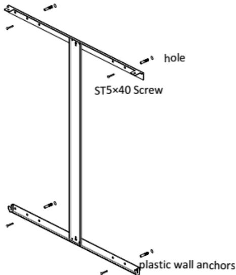
**Note:** For 890E and 1500E, mark and drill four holes on the wall using this kind of wall bracket as a template and fix the wall mount bracket onto the wall with ST5\*40 screws.
