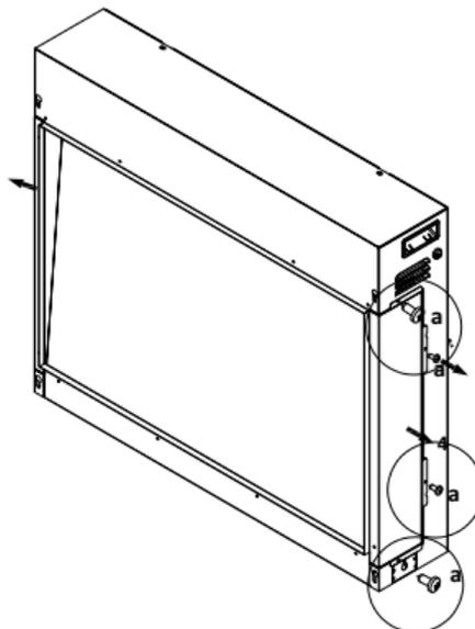
5.5c Put the fire box onto the wall bracket and then fix with two fixing screws of the wall mount brackets on the top of the fire box. Remove the front glass and arrange the fuel bed as described in 5.4c and 5.4d.
