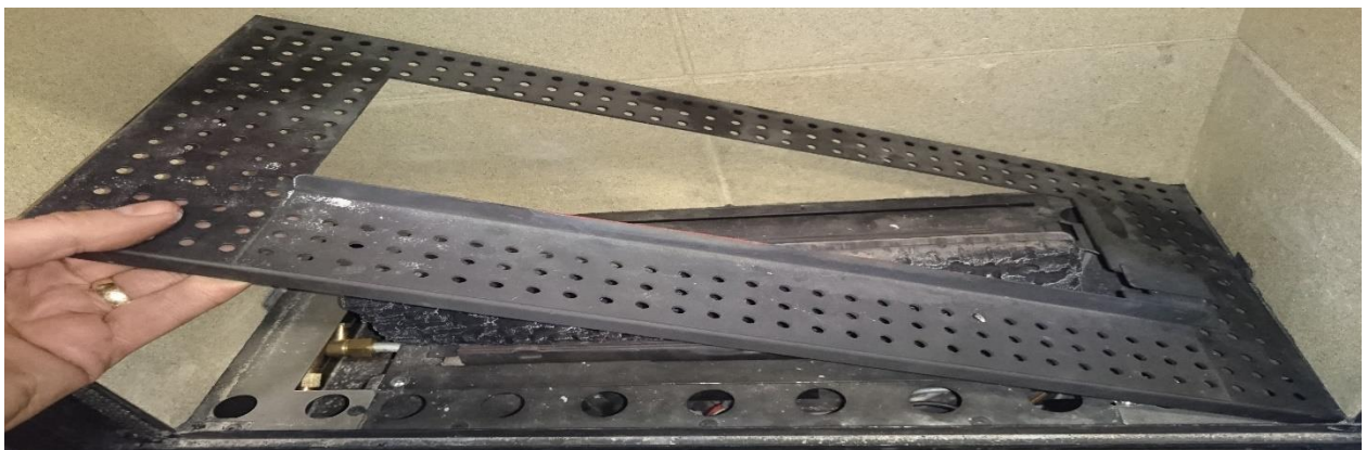
Slide air tray in to place make sure it is central and sitting flat
