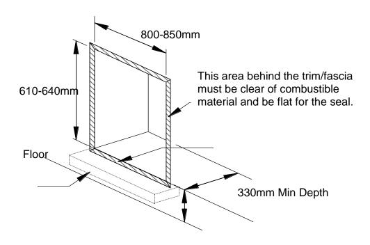
The front face and the base of the fire opening must be flat to ensure that a good seal is formed between the rear and base of the appliance and the chimney to avoid any reduction of natural draught.
