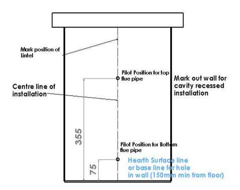
• Using 125mm (5") core drill cut two holes following the pilot holes. Drill from the outside through to the cavity to give a good finish on the outside.
