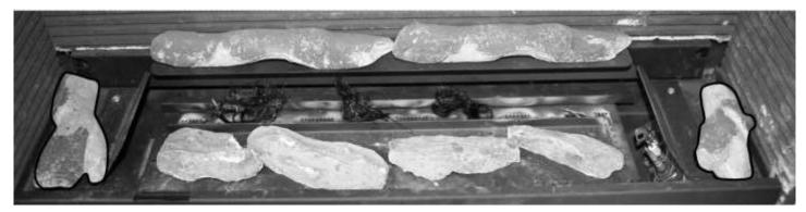
• Place the next two large shapes LH and RH of the burner bar as shown.
