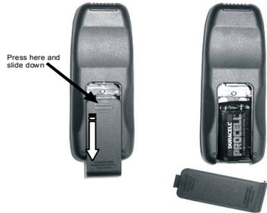
FIGURE 8 HANDSET BATTERY REPLACEMENT
