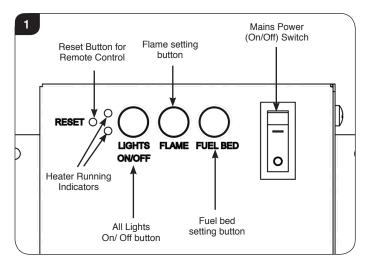
Note: The appliance will lose the memory for the light functions when the switch is set to the Off Position or the remote runs out of power.
