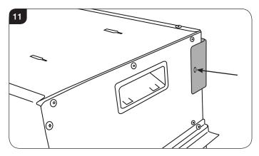
4.13 Fasten the two lower fixing bracket to the 2 fixing points on the underside of the appliance and secure to the wall, see Diagrams 12 & 13.
