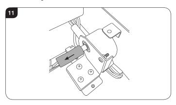
7.5 Withdraw the spindle from the left hand bracket, see Diagram 12.
