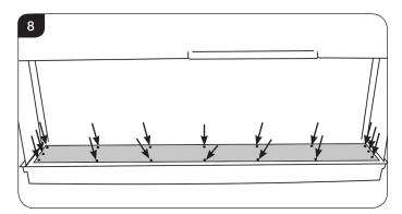
6.3 The flexible fuel bed can now be lifted out of the appliance.
