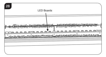
12.4 The LED boards are coupled together at the end of each board and held in place by clips, see Diagram 29.
