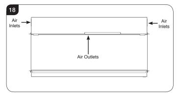
Dust build-up can inhibit efficient performance of the fan and lead to the safety cut-out operating.
