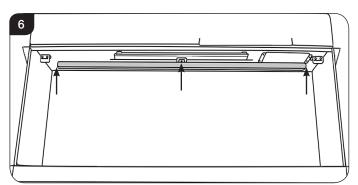
5.3 Carefully lower the LED Light Bar and disconnect the cable from the right hand side, see Diagram 7.
