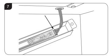
NOTE: When replacing the LED Light Bar ensure that the central tab is positioned at the front of the firebox.
