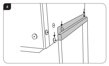
3.4 Fit the bottom Corner Side Glass Retainer bracket ensuring both screws are replaced, see Diagram 5.
