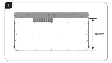
4.6 To prepare the installation measure the distance from floor level and using a spirit level draw a line 485mm higher than the intended position of the bottom of the appliance. NOTE: If fitting a Trento surround add 30mm to the bottom of the appliance.
