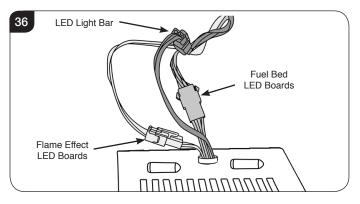
15.7 Replace in reverse order. Ensure all the leads are reconnected following the previous orientation.
