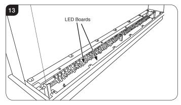
8.3 The LED boards are coupled together at the end of each board and held in place by clips, see Diagram 14.
