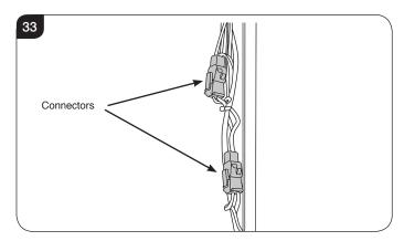
14.6 Replace in reverse order, ensuring the cable ties are replaced.
