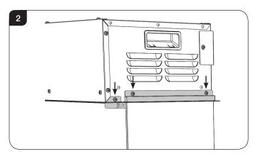
3.2 Remove the 2 Screws securing the lower bracket, see Diagram 3.
