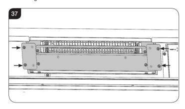
16.3 Carefully lower the Heater Assembly. This will require a slight tipping motion to clear the edge, see Diagram 38. NOTE: The Heater Assembly has wires attached.
