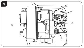
5.6 Remove the 2 screws securing the valve to the support bracket and withdraw the valve.
