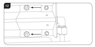
8.4 Undo the 14mm lock nut that holds the pipe to the injector, see Diagram 13.
