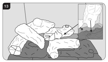
6.7 Sit the first hole in the bottom of the left hand side of Log K on the stud of Log H and secure by fitting the middle hole on the right hand side over the stud in the fuel bed by the burner port, see Diagram 14.
