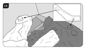
6.8 Log K should rest on the flat plain behind the stud for the Log arrangement to be complete, see Diagram 15.
