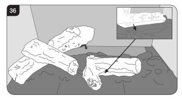
7.15 Rest log D on the raised stud on log C. The rear of the effect should rest against the back liner, see Diagram 37.
