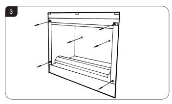
3.8 Slide the inner box away from the outer box by pulling it forward, see Diagram 4.
