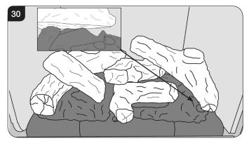
7.9 Lay Embaglow over the small ports in the base of the burner tray. This will create a glowing effect when the appliance is lit, see Diagram 31.
