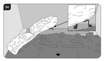
7.13 Place log B on top of log A. There is a hole on the underside of log B which fits over the raised stud in log A to secure in place, see Diagram 35.
