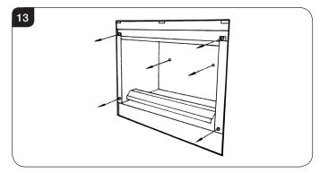
3.22 Replace the burner module and secure in position. Replace the ceramic panels as detailed in Replacing Parts, Section 2.
