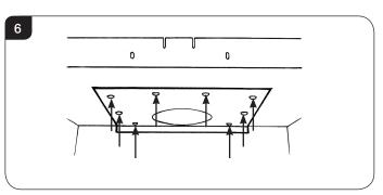
3.12 Pull the liner through the hole in the top of the outer box and attach it to the flue spigot plate using the clip provided. Tighten the clip securely, see Diagram 7.
