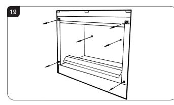
11.10 Slide the inner box away from the outer box by pulling it forward, see Diagram 20.
