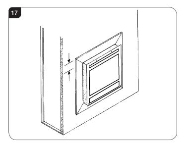
4.8 Push the cassette back into its final position and connect the flue system, gas and electric services using the openings in the side of the chimney breast for access. Following commissioning complete the sides of the chimney breast, see Diagram 18.
