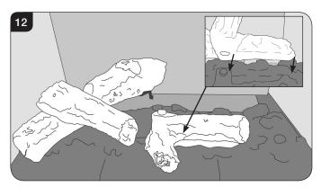
6.6 Rest Log I on the raised stud on Log H. The rear of the effect should rest in the groove at the back of the burner tray, see Diagram 13.
