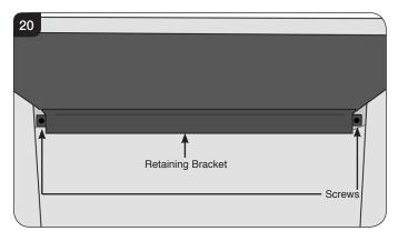
6.3 Slide the back liner panel over the bracket in the base of the firebox and stand upright against the back of the appliance, see Diagram 21.
