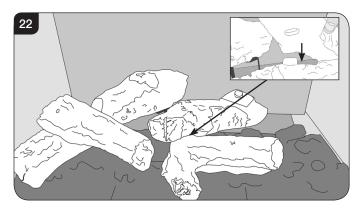
6.16 Sit the hole in the bottom of Log E on the stud of Log D and rest the other end in the groove in the fuel bed by the burner port, see Diagram 23.
