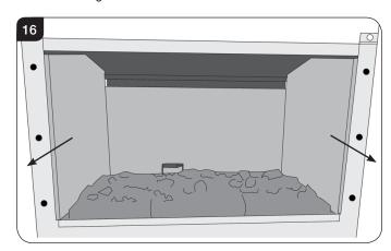
11.5 Remove the bracket in sat the back of the firebox and carefully remove the back panel, see Diagram 17.
