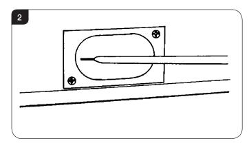
2.3 When installing the appliance into a combustible enclosure, ensure all the clearances are observed. Refer to Site Requirements, Section 4.
