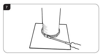
3.13 Secure the flue spigot plate to the inside top surface using the 8 screws provided, see Diagram 6.
