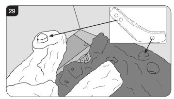
7.8 Log K should rest on the flat plain behind the stud for the Log arrangement to be complete, see Diagram 30.
