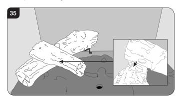
7.14 Place log C on the centre of the burner tray. There is a raised stud in the fuel bed which securely locates the left hand side of the log in place whilst the right hand side rests in the channel to the right hand side of the air cutout in the fuel bed, see Diagram 36.
