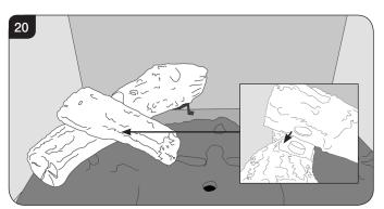
6.14 Place log C on the centre of the burner tray. There is a raised stud in the fuel bed which securely locates the left hand side of the log in place whilst the right hand side rests in the channel to the right hand side of the air cutout in the fuel bed, see Diagram 21.
