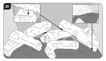
7.17 Lay Embaglow over the small ports in the base of the burner tray. This will create a glowing effect when the appliance is lit, see Diagram 39.
