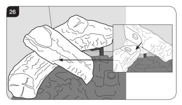
7.5 Place Log H on the centre of the burner tray. There is a raised stud in the fuel bed which securely locates the log in place. The right hand side rests on the raised section at the end of the air cutout, see Diagram 27.
