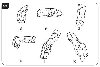
7.2 Place log A on the left hand front of the burner. The log will fit over the raised stud and into the raised stud and into the groove in the burner tray, see Diagram 24.
