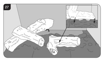
7.6 Rest Log I on the raised stud on Log H. The rear of the effect should rest in the groove at the back of the burner tray, see Diagram 28.
