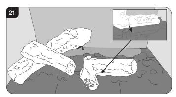
6.15 Rest log D on the raised stud on log C. The rear of the effect should rest against the back liner, see Diagram 22.
