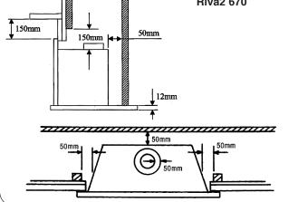
It is recommended that a marble slip or similar material is used when fitting cassette fireplaces into a plastered surface, in order to allow for heat dissipation. Also allow adequate time for newly plastered areas to dry out. Rapid drying can create cracks. If in doubt, seek the advice of a professional plasterer.
