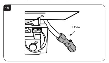
5.2 Connect a suitable pressure gauge to the test point located on the inlet fitting and turn the gas supply on. Light the appliance and check all gas joints for possible leaks. Turn the appliance to maximum and check that the supply pressure is as stated on the databadge. Turn the gas off and replace the test point screw, turn the gas on and check the test point for leaks.
