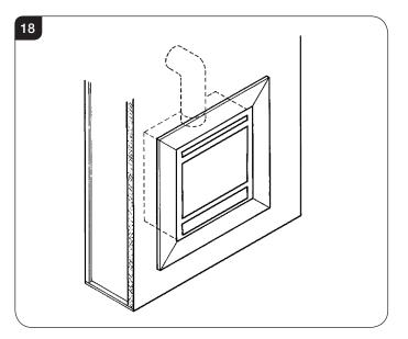
4.9 A removable access hatch must be left in the side of the chimney breast for future servicing and inspection of the appliance.
