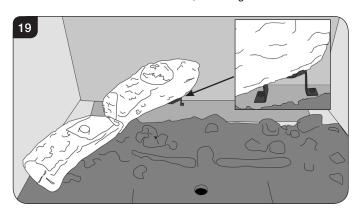
6.13 Place log B on top of log A. There is a hole on the underside of log B which fits over the raised stud in log A to secure in place, see Diagram 20.
