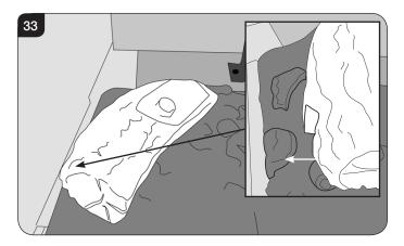
7.12 Place log F behind the first log and locate the rear of the log on the metal bracket. The log should rest between the lip of the bracket and the rear liner, see Diagram 34.
