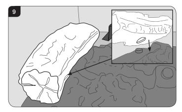
6.3 Place Log F behind the Log A on the flat plain and locate the rear of the log on the metal bracket. The log should rest between the lip of the bracket and the rear liner, see Diagram 10.
