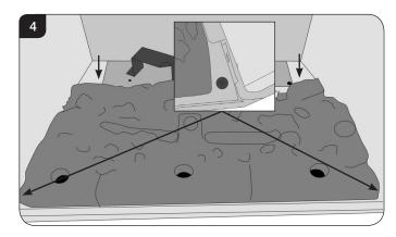
2.11 Carefully remove the fuel bed and place safely to one side.
