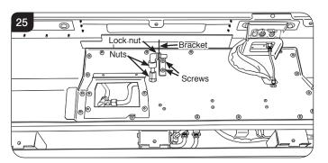
11.3 Remove the 2 screws and the bracket.
