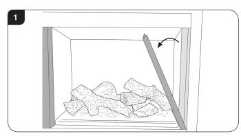
2.3 Lift out the bottom Slotted Trim, see Diagram 2. Note the orientation of the metal shield for reassembly.
