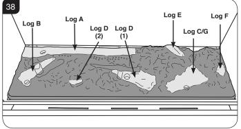
11.4 Place log C (Nat Gas) or G (LPG) on the right hand side of the burner, see Diagram 20. The log will rest on the flat location point shown in Diagram 39.
