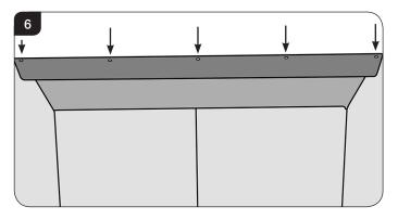
3.3 The Baffle can now be removed by lowering the front edge and pulling forward through the front of the appliance. TAKE CARE NOT TO DAMAGE THE SIDE PANELS.
