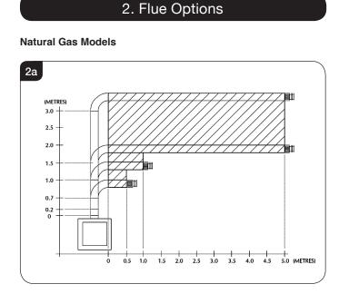
Start of bend to centre line of horizontal flue 170mm. Centre line of vertical flue to end of bend 220mm.
