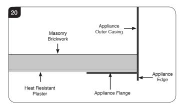
7b.6 The subframe for the decorative front can now be fitted by following the instructions supplied with the Front. NOTE: THE SUBFRAME MUST SIT FLUSH TO THE WALL LEVEL WITH THE APPLIANCE FLANGE.
