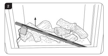
2.4 Disconnect the battery lead from the Battery Pack attached to the lower slotted trim, see Diagram 3.
