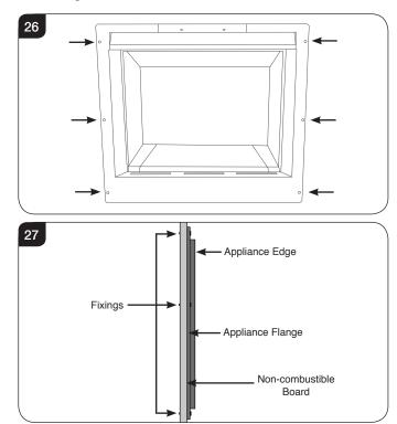
8a.10 Fit non-combustible board to the board around the appliance, see Diagram 28. Ensure distances to combustibles are observed, see Diagram 21.
