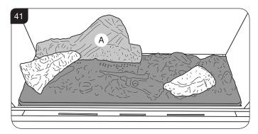
11.7 Position the right hand end of log D on the flat location plain on the burner, as shown in Diagram 38, Log D (1). Rest the left hand end of the log across log B, see Diagram 42. Ensure that the front branch rests in the location point on the burner, as shown in Diagram 38, Log D (2).
