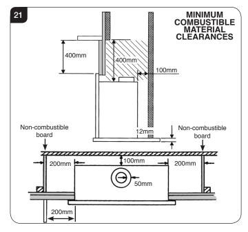
8.2 DISTANCE TO NON-COMBUSTIBLE OR COMBUSTIBLE MATERIAL TO CREATE ENOUGH CLEARANCE FOR THE TOP
