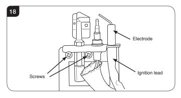
IMPORTANT The Ignition Lead and the Thermocouple need to be removed at the same time regardless of which needs to be replaced.
