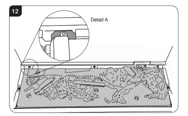
4.6 Slide the Burner Tray to the right, pull slightly forward and lift from the back. Carefully remove through the front of the appliance. Place carefully to one side.
