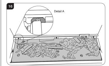
6.3 Slide the burner unit to the right, pull slightly forward and lift from the back. Carefully remove through the front of the appliance. Place carefully to one side.
