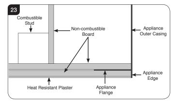
NOTE: If metal studwork is used, there is no need to fit non-combustible board to the face of the construction, see Diagram 24.
