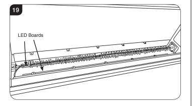
9.3 The LED boards are coupled together at the end of each board and held in place by clips, see Diagram 20.
