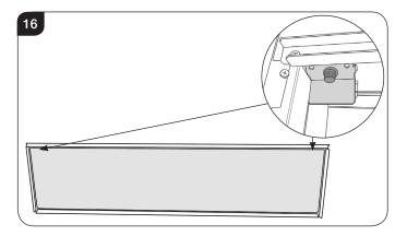
3.7 Supporting the glass, loosen and remove the 2 clamps. These can be unscrewed using just finger tips.
