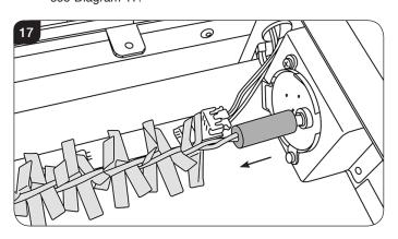
8.5 Withdraw the spindle from the left hand bracket, see Diagram 18. The spindle may need to be tilted to be removed from the location bracket.
