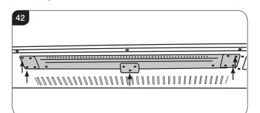
17.4 Carefully lower the Heater Assembly. This will require a slight tipping motion to clear the edge, see Diagram 43. NOTE: The Heater Assembly has wires attached.
