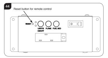
Resetting of the remote control is necessary if the appliance operates wrongly due to external interference signal and the remote control is not in use.
