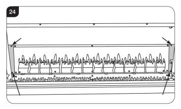
Note: When refitting the brackets the folded tab must be located at the top, see Diagram 25.
