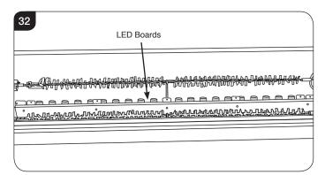
13.4 The LED boards are coupled together at the end of each board and held in place by clips, see Diagram 33.
