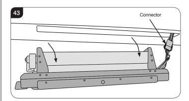
17.5 Carefully feed the wires over the between the Heater Assembly and Power Unit apertures.
