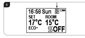
2b.11 Hold the ← button for 6 seconds to enter the daily heating setting.
