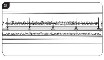
NOTE: When refitting the shield ensure that the lip curves down and towards the back. It will be necessary to lift the shield slightly to align the screws. Refit the screws from inside out.
