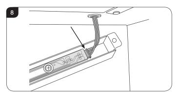
NOTE: When replacing the LED Light Bar ensure that the central tab is positioned at the front of the firebox.
