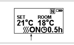
Note: It is normal for the fan heater to stop running for periods of time. This happens if the room temperature is higher than the temperature set on the control.
