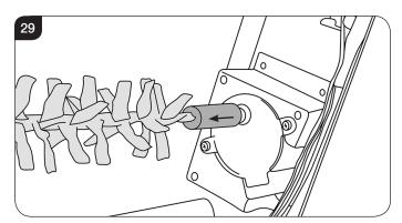
12.5 Withdraw the spindle from the left hand bracket, see Diagram 30. The spindle may need to be tilted to be removed from the location bracket.
