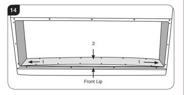
7.6 Press the fuel bed flat so that the front locates under the front lip, see Diagram 14 (2). Adjust the position so that the screw holes line up.
