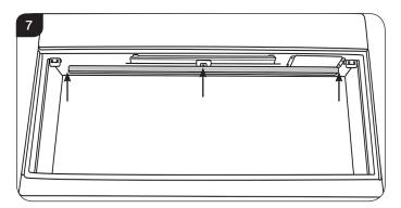
5.2 Carefully lower the LED Light Bar and disconnect the cable from the right hand side, see Diagram 8.
