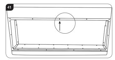
17.3 The Heater Assembly is now held in place by 5 screws at the top of the firebox.Supporting the Heater Assembly remove the screws, see Diagram 42.
