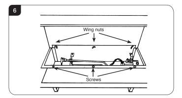
4.11 Take the separated firebox through the fireplace opening. Secure the four rear and three lower holes using rawl plugs and screws provided, see Diagram 7.
