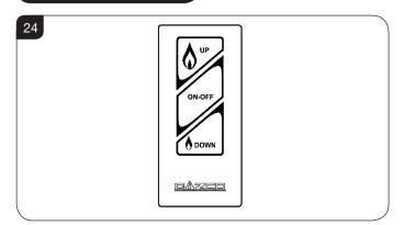
8.4 **To light the aplliance** press the ON-OFF button (up to 30 seconds).
