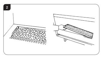
1.8 Empty the fuel effect into a suitable container and place the tray down.
