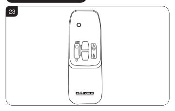
8.1 To light the appliance press the LOWER section of the LEFT hand button and the UP button simultaneously. An audible beep will be heard (the lighting sequence can take up to 30 seconds).
